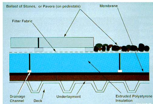
A Protected Roof Membrane Assembly (PMRA) differs from a conventional roof design in that the membrane is placed under the insulation layer, maximizing membrane life by protecting it from temperature extremes, freeze/thaw cycles, UV degradation, and traffic wear. A PMRA begins with the application of the EPDM membrane, followed by the XPS boards, the protective scrim, and finally the ballast. Extruded polystyrene foam is the only type of insulation recommended for use in a PRMA system because it
