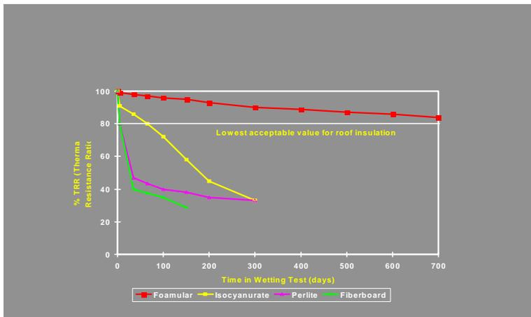
**Figure 1.** Data from “New wetting curves for common roof insulations” Wayne Tobiasson, Alan Grestorex and Doris Van Pelt, U.S. Army Corps of Engineers Cold Regions Research and Engineering Laboratory Hanover, New Hampshire
