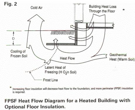
FPSF Heat Flow Diagram for a Heated Building with Optional Floor Insulation.
