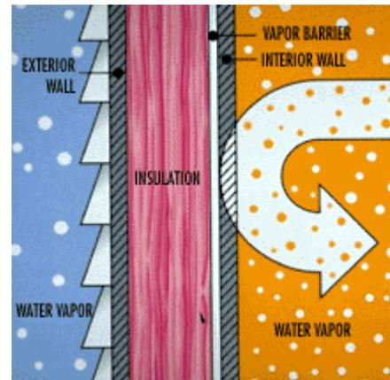
Unlike many other types of sheathing, XPS does not have to rely on facers or laminates to obtain compressive strength or achieve its ability to resist water moisture intrusion. Therefore, it is an excellent choice for ensuring a building's envelope will be properly sheathed and assure that its subsequent performance will not be compromised during installation of the sheathing due to nails, glue and other materials.
