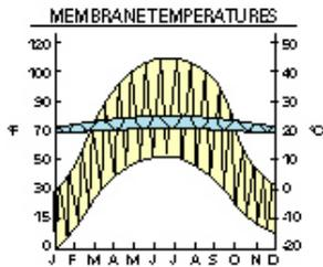
PMR roof (blue line) – the membrane temperature remains relatively constant.
