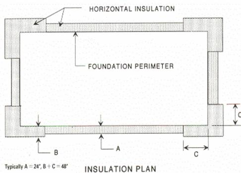
FPSF design parameters for heated buildings using the simplified design procedure.
