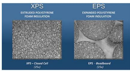
**Figure 2:** Cellular structure differences between extruded and expanded polystyrene (XPS and EPS) foam insulations. Images
