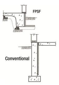
*Figure 3:* At the top left, a frost-protected shallow foundation (FPSF); at bottom right, a typical foundation. Image courtesy U.S. Department of Housing and Urban Development
