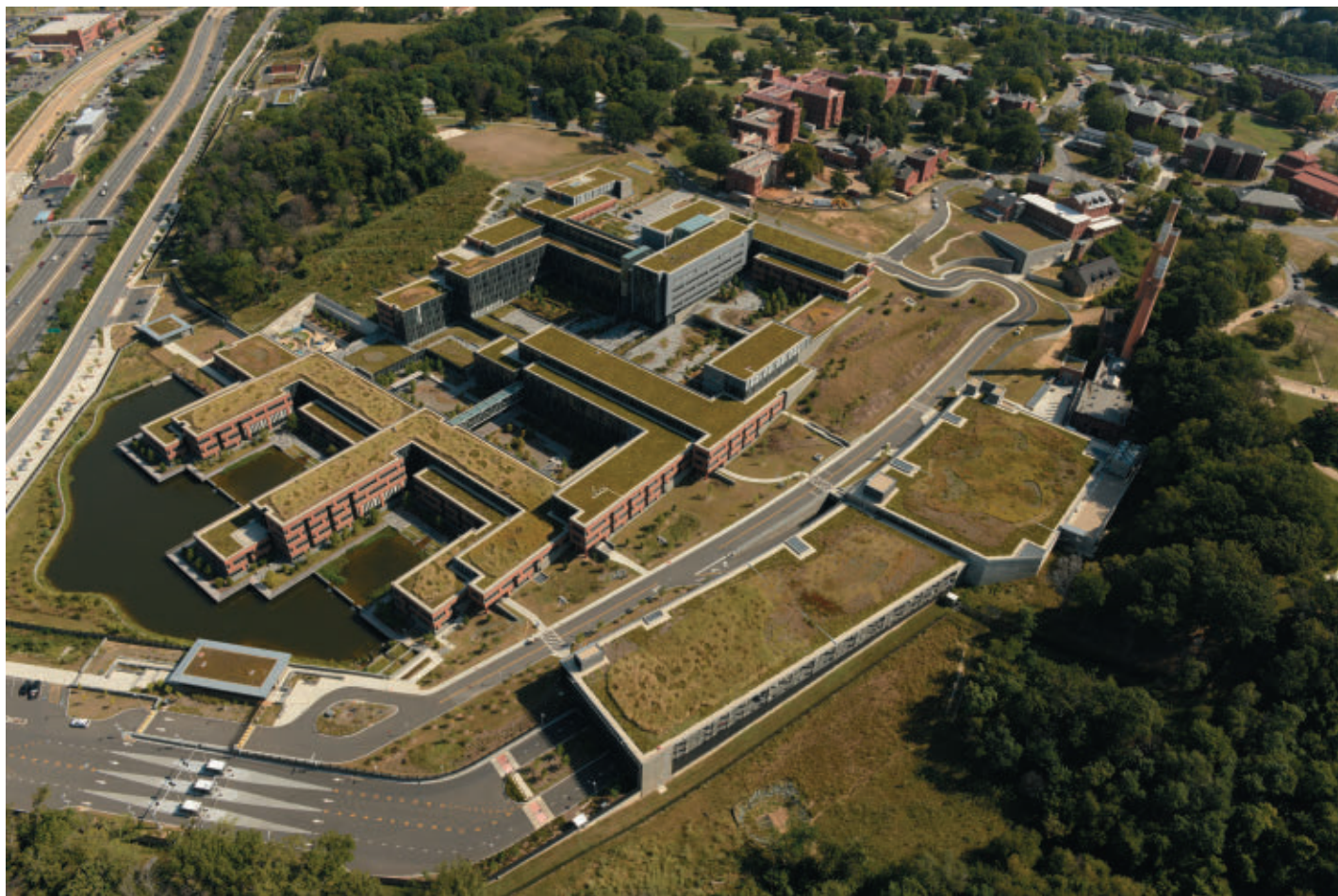
Figure 7. Aerial view of US Coast Guard Headquarters. XPS insulation must resist compressive loads from the weight of vegetative or “green” roofs. Note: The appearance of US Department of Defense (DoD) visual information does not imply or constitute DoD endorsement. EPS = expanded polystyrene; XPS = extruded polystyrene.
