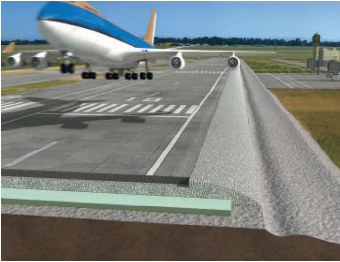
Figure 2. Rigid, cellular polystyrene foam boards are often installed beneath airfields in cold climates.
